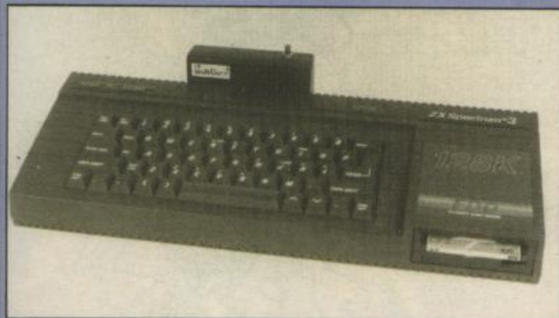
▶ A pawn in the pirate war: Romantic Robot's Multiface 3 offers cassette-to-disk transfer, but it could be thwarted by +3 programs
